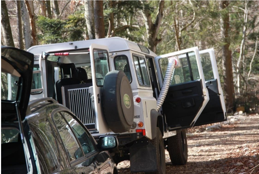
Fig. 2.4.3. Outside air is caught by an external quiet fan (see tube) to ventilate the transport box to prevent hyperthermia during transport.
