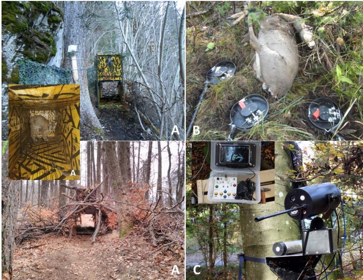
Fig. 2.4.1. Capture systems. A) box traps installed on forest roads, B) Foot snares, C) tele-guided dart gun (MICS).
